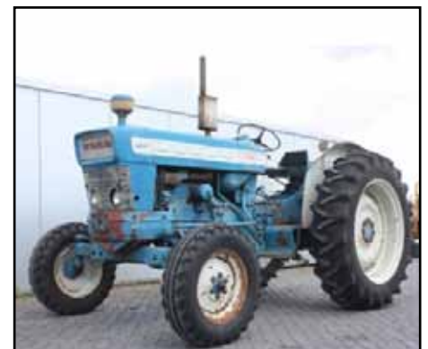
The fluted bonnet, canister type oil filter and old style grill identify this as an early Ford 5000.
