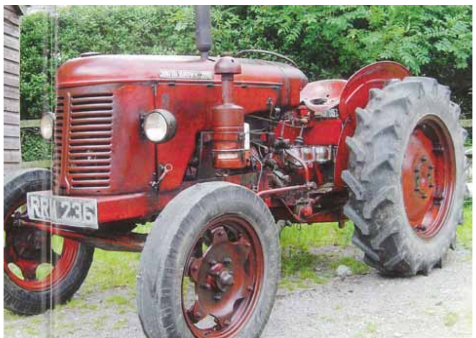
this David Brown 25D has been carefully conserved by its owner with a coat of light oil to protect its original finish
