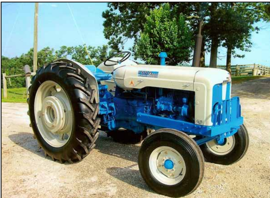
The fluted bonnet, canister type oil filter and old style grill identify this as an early Ford 5000.
