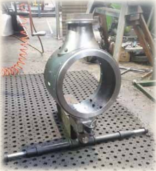
September - Front axle and perch bracket and chimney saddle test fitted to the smokebox.
